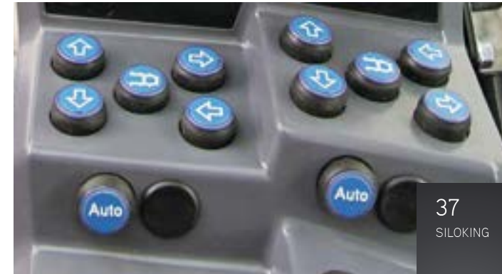
The discharge conveyors are controlled simply by pushing a button from the driver's cab.
