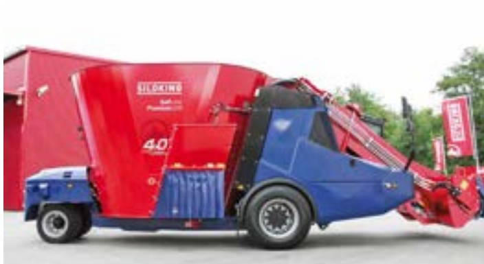
Discharge door at front right.
