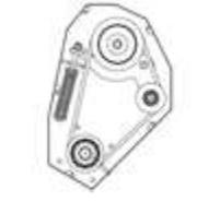
AUTOMATIC BELTS TENSIONER The automatic tensioning system as well as allowing constant power transmission reduces belts wear.
