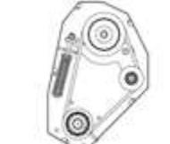
AUTOMATIC BELTS TENSIONER The automatic tensioning system as well as allowing constant power transmission reduces belts wear.
