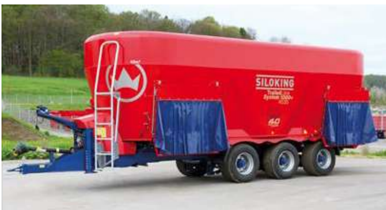
TrailedLine 4.0 System 1000+ 4535-40 with heavy-duty discharge doors.
