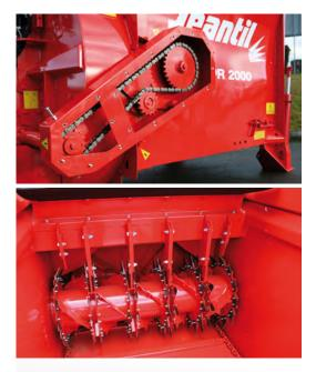
**High-performance shredder** The shredder with knives supplies the turbine with all types of products regularly. The mechanical drive ensures a high power shredding.
