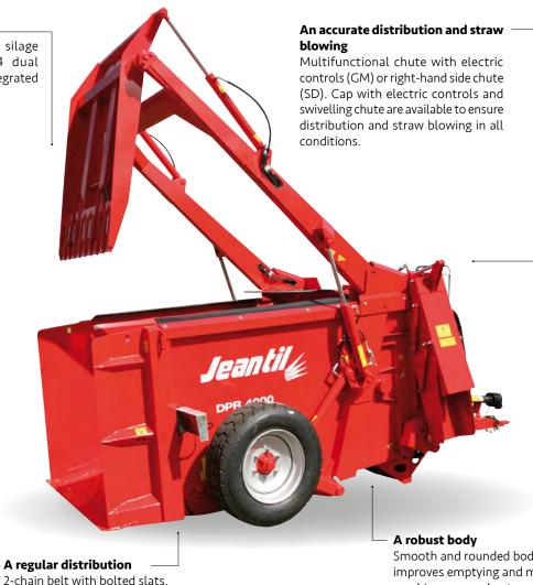
Smooth and rounded body which improves emptying and makes the machine more robust.
