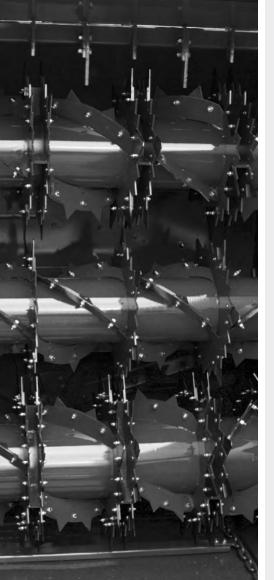
BASIC and SMART proportional electric controls drive the moving floor with precision. Thanks to the SMART controls, the drive of the shredders regulates the moving floor speed depending on the distributed product.
