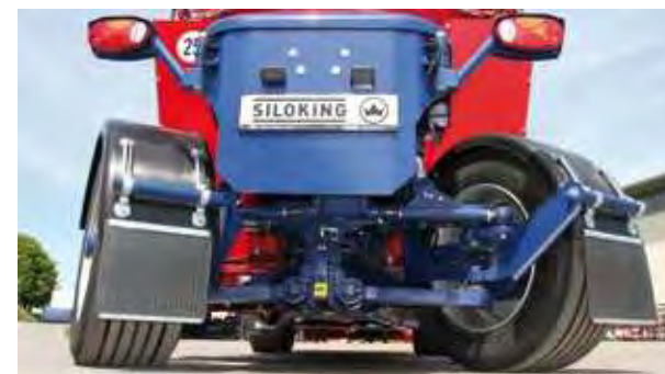
Standard with SelfLine 4.0 Premium 2215-22 : The professional independent wheel suspension has high load-bearing capacity and is very wear-resistant.
