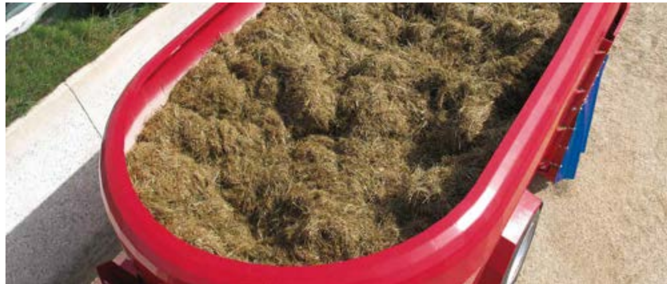
The rounded FlowPlus hopper ring takes the feed from the top back down into the mixing process, thus ensuring clog-free working, even when processing round bales.
