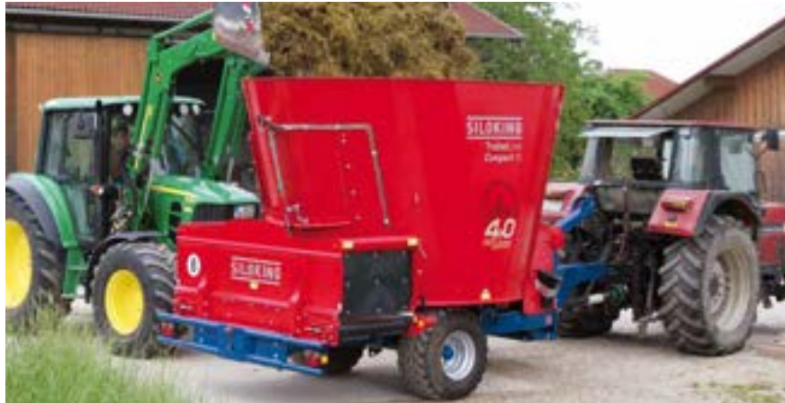
The robust underrun protection with integral lighting protects humans, animals and the machine in an optimal way by day and by night.
