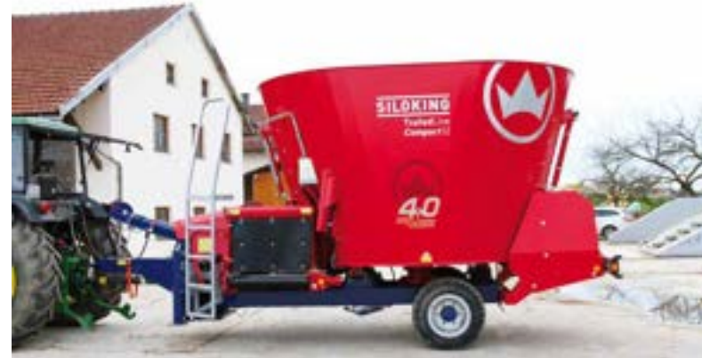
Cross conveyor belt at front and discharge door at rear centre.
