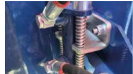
Hydraulic shift for 2-speed gearbox.
