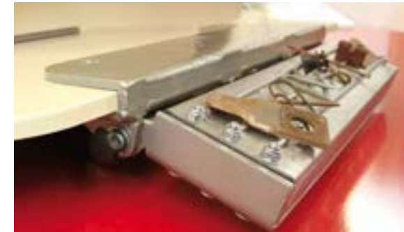
Heavy-duty neodymium magnet in perfect position.
