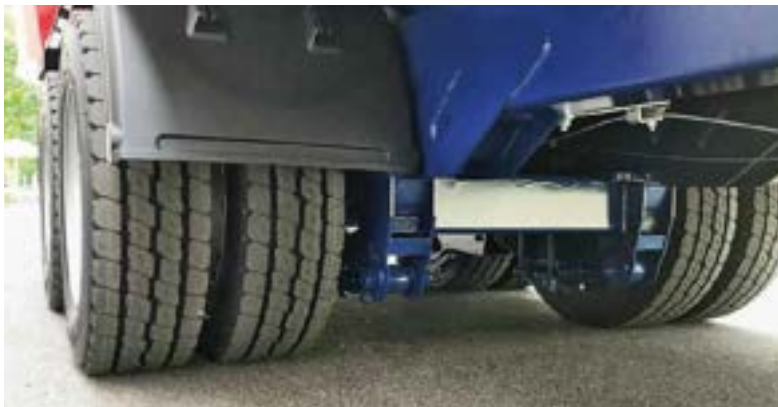
Heavy-duty tandem axle 32 t with twin tyres for use only on the farm premises (optional).
