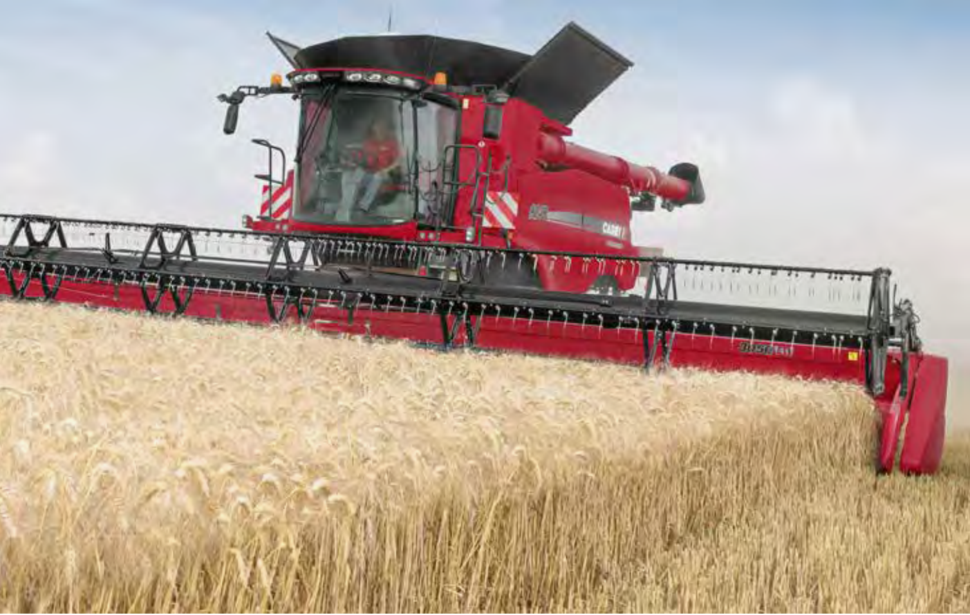
Valuable Benefit: Tines reach 7,5 cm below the knifebar to lift up crop and reduce knife damage.
