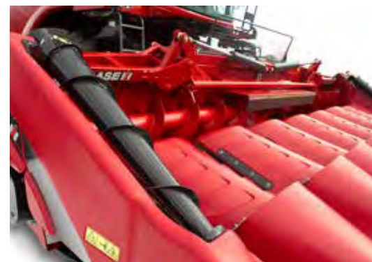
The layed crop spiral auger and the grain retention louvers - Perfect design for no losses
