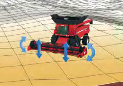
Case IH Terrain Tracker technology ensures an exact cutting height is maintained across the most uneven of ground.
