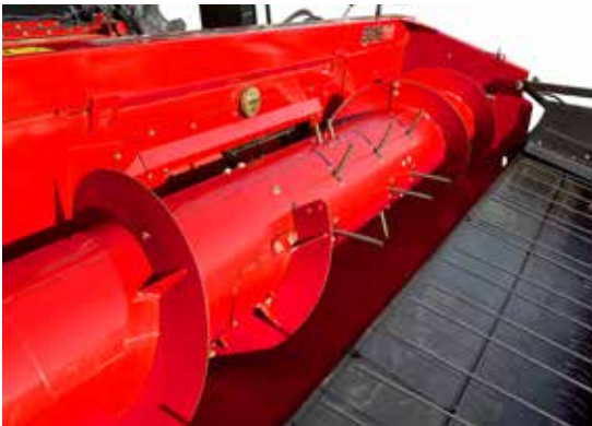
Large diameter auger to feed high density swaths into combine
