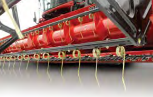
Valuable Benefit: Tines reach 7,5 cm below the knifebar to lift up crop and reduce knife damage.
