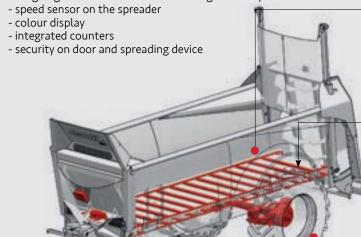
Control of the rotation of the beater for safety on the moving floor
