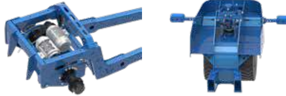
Hydraulic suspension at the front and rear
